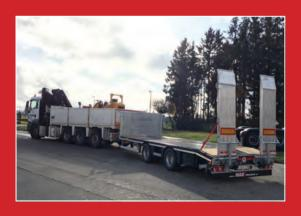
MAX Trailer, 2 axle draw bar, spring loaded alu ramps, option for side boards
