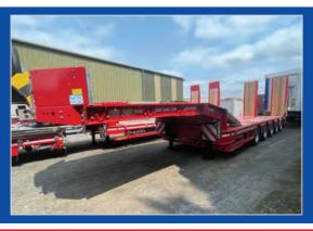
Faymonville 5 axle step frame low loader, 70ton payload, extendable by 6m, double flip ramps, marker boards, out rigger timbers, front lift axle, 3 steer axles, available in stock
