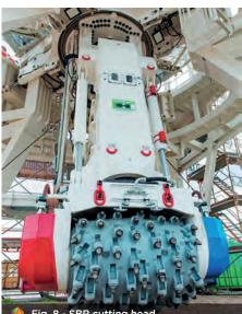
Fig. 8 - SBR cutting head.
