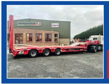
**NEW FAYMONVILLE MULTIMAX** 66ton gross trailer weight, 9ft wide, double flip ramps, hydraulic rear legs, out riggers, option for extendable bed.
