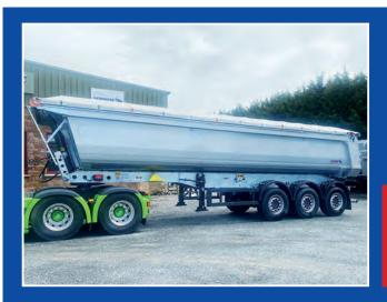
SCHMITZ TIPPING TRAILERS 9.6m, galvanised chassis, hardox steel body, electric cover, sealed tail board, metallic silver body.
