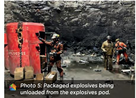
Photo 5: Packaged explosives being unloaded from the explosives pod.
