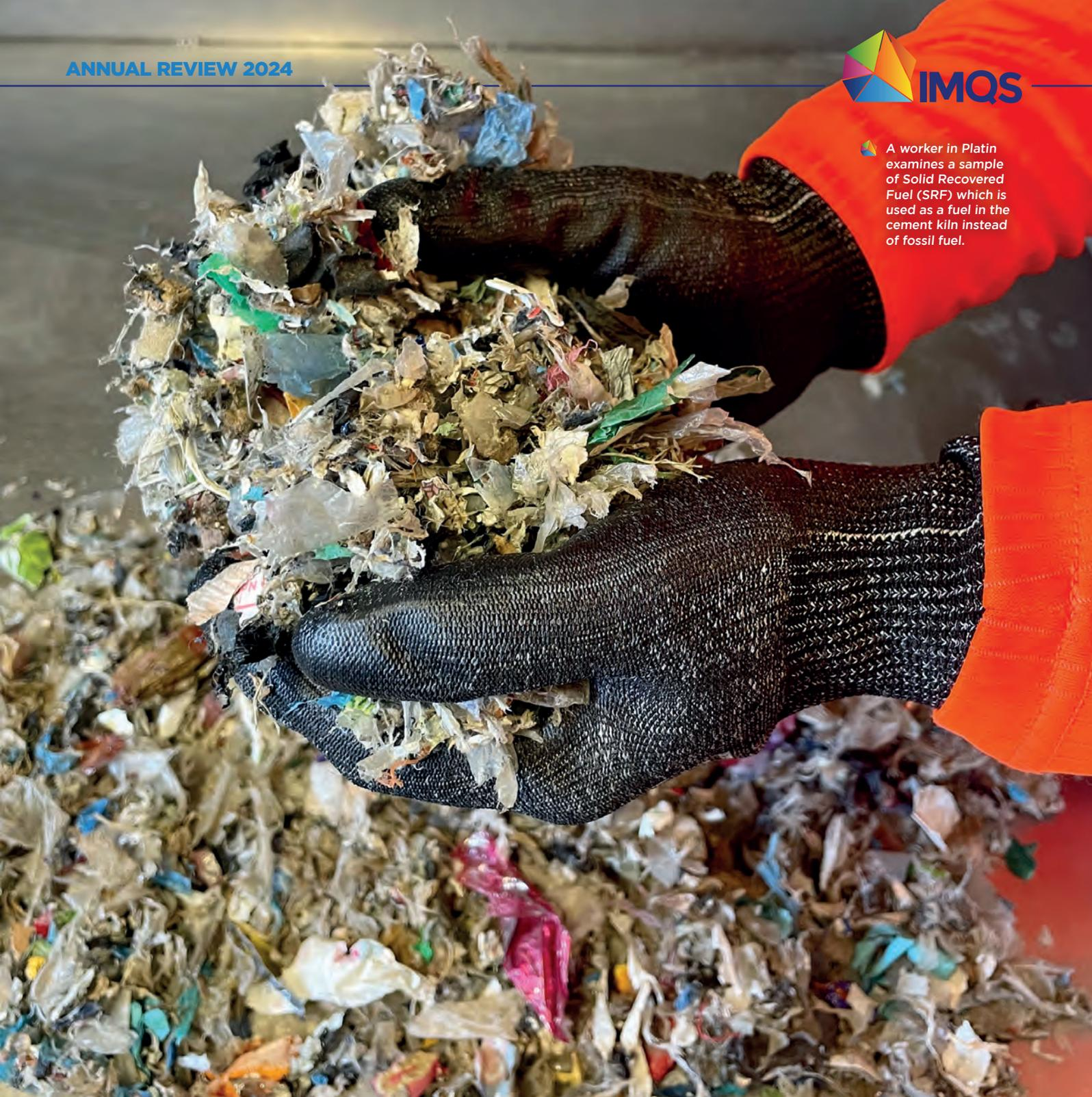
released from the combustion of the SRF, the non-combustible or mineral fraction, in this case the aluminium combines with other raw materials to form some of the minerals required in clinker.
