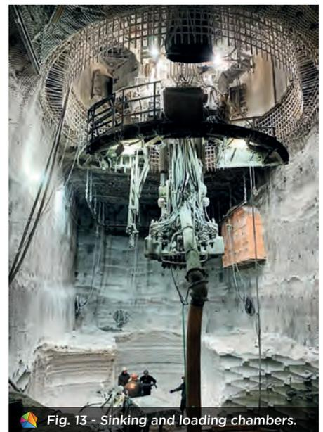
Fig. 13 - Sinking and loading chambers.
