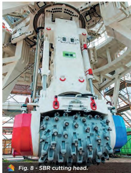
Fig. 8 - SBR cutting head.
