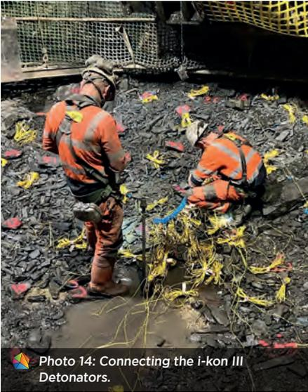
Photo 14: Connecting the i-kon III Detonators.
