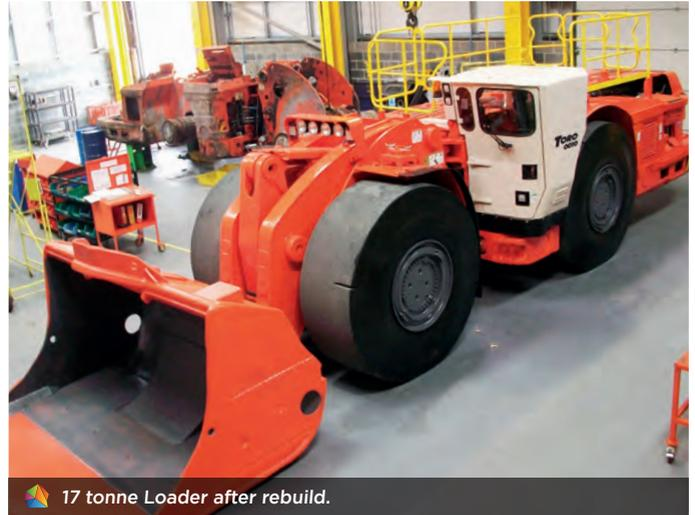
17 tonne Loader after rebuild.
