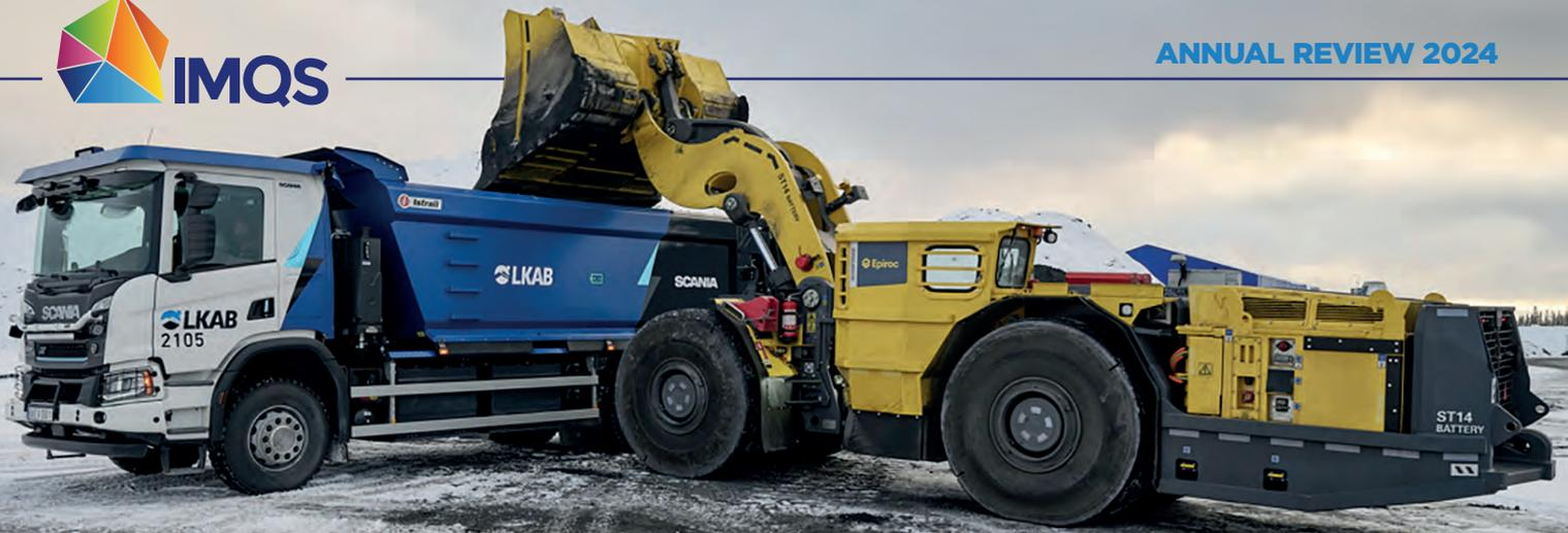
Mine electrification in action – the Epiroc ST14B battery-powered LHD loading the Scania P450 battery-powered truck at Malmberget Mine. (Photo LKAB).
