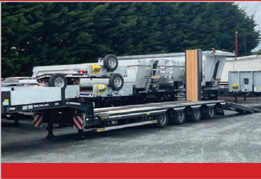
Faymonville 4 axle step frame low loader Hydraulic widening bed, 2.54m bed widens to 3.2m at the push of a button, Extendable in length by 6.5m, Double flip ramps with hydraulic side shift, Hydraulic rear support legs
