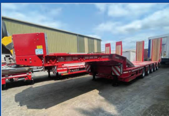
Faymonville 5 axle step frame low loader, 70ton payload, extendable by 6m, double flip ramps, marker boards, out rigger timbers, front lift axle, 3 steer axles, available in stock
