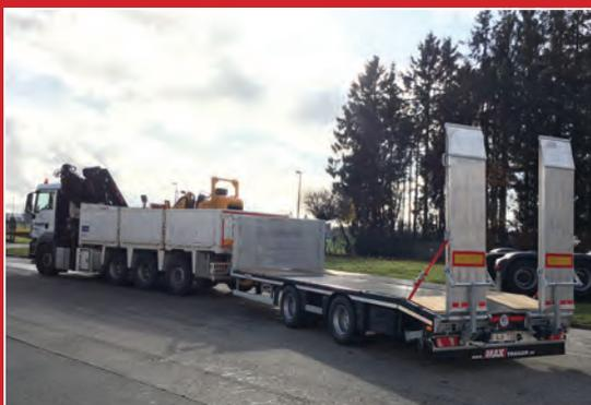
MAX Trailer, 2 axle draw bar, spring loaded alu ramps, option for side boards
