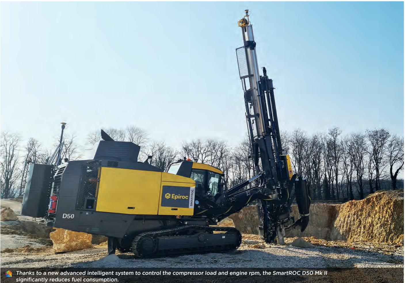
Thanks to a new advanced intelligent system to control the compressor load and engine rpm, the SmartROC D50 Mk II significantly reduces fuel consumption.
