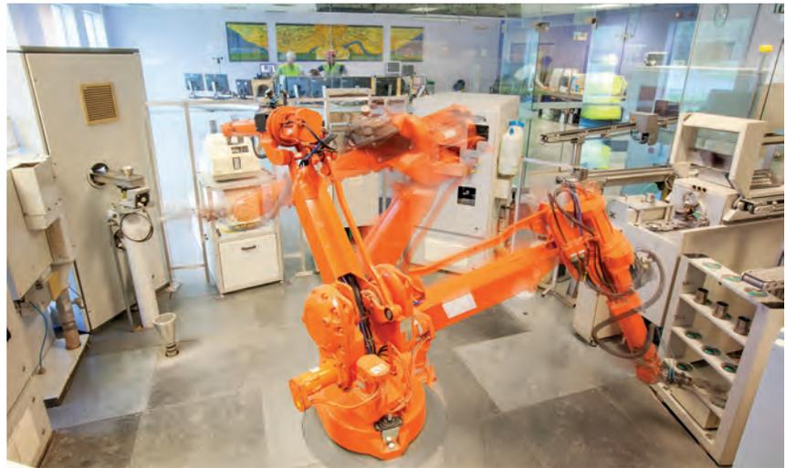
**Modern high-tech cement production, this is a composite photograph of an autolab robot in action beside the main plant control room. Samples are automatically delivered to the autolab from throughout the plant for testing and the results pass directly into the central control system. Photo credit; DAK Photography**
