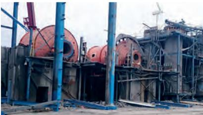
Fig. 5 – The SAG and Ball mill exposed and awaiting removal.
