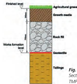
Fig. 19 – Section of the TMF cap.
