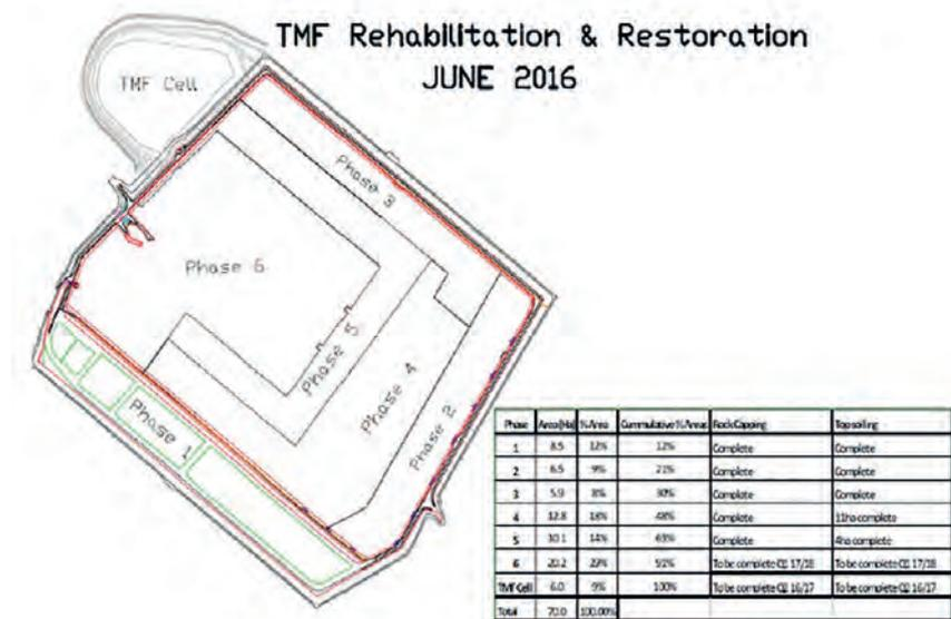
Fig. 25 – Schedule for remaining phases of TMF (plan for completion mid 2017).
