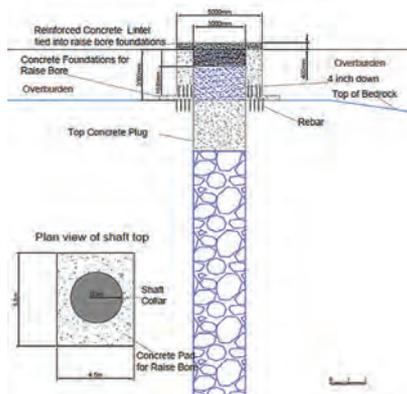
Fig. 8 – Typical fill detail for a vertical shaft.
