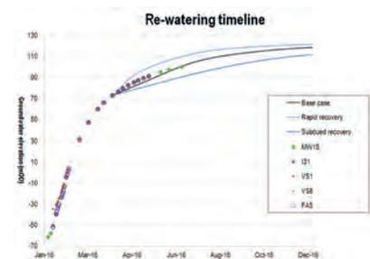
Fig. 2 – Rate of rise of water within the Mine.
