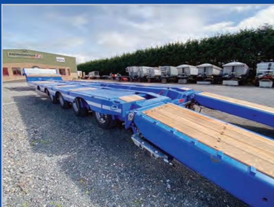
New Faymonville 4-axle hydraulic widening bed low loader, extendable in width from 2.54m to 3.2m at the push of a button, also extendable in length, double flip hydraulic ramps, rear steer axles, hydraulic rear legs, full spec. In stock available immediately.
