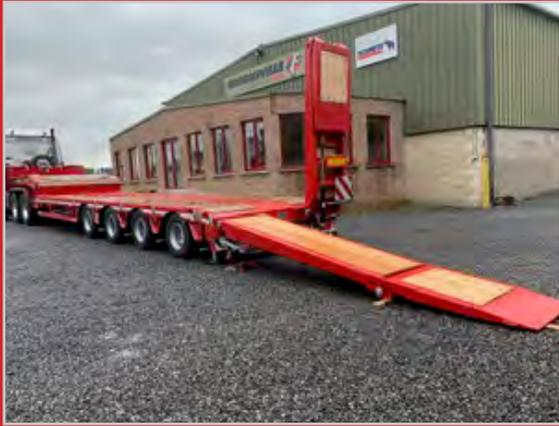
New Faymonville 4 axle step frames in stock and available on short delivery times. Extendable and fixed bed, 9ft wide, single or double flip ramps.
