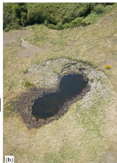
**(a)** Aerial photos of Maidenmount mine: (a) UAV derived ortho-photograph and (b) a close up of the crown hole at Maidenmount, acquired in 2016.
