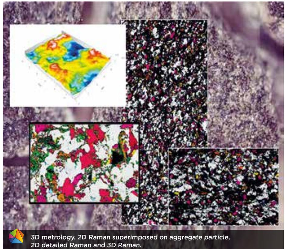
**3D metrology, 2D Raman superimposed on aggregate particle, 2D detailed Raman and 3D Raman.**
