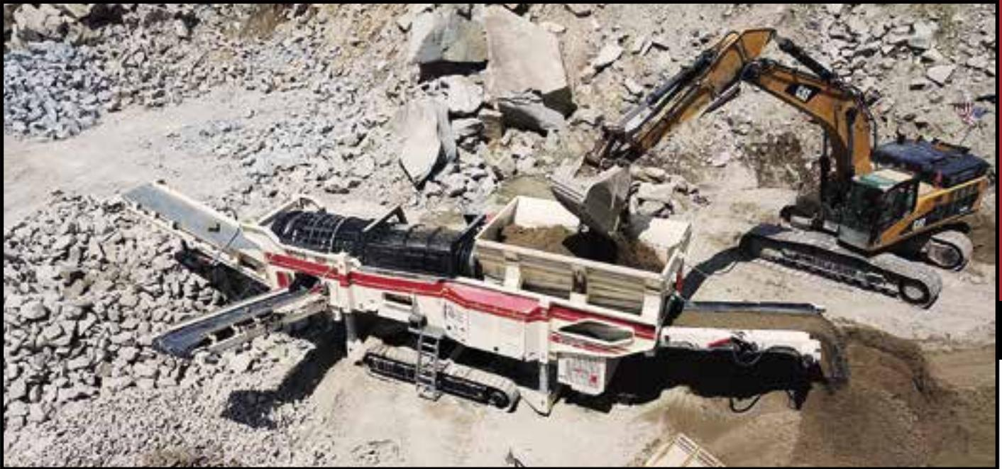
Trommel technological advances present in our M412 and M515 range have made huge savings in terms of fuel efficiency and low wear costs when dealing with overburden.
