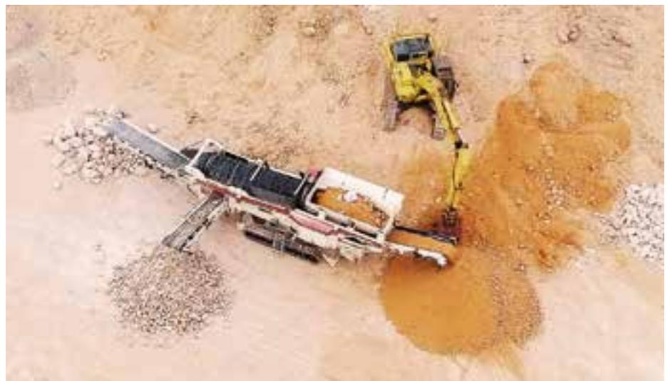
of soil and rocks. The soil has a high plasticity clay content which is stuck to the rocks. This type of clay clumps together instead of breaking up and is very problematic for regular vibratory screeners. The vibrating action liquifies the clay and makes it stick to the openings and blocks up the screens. Also, the rocks found in this mixture are as large as 800mm and are too big for regular vibratory screeners or recycling tromeels.
