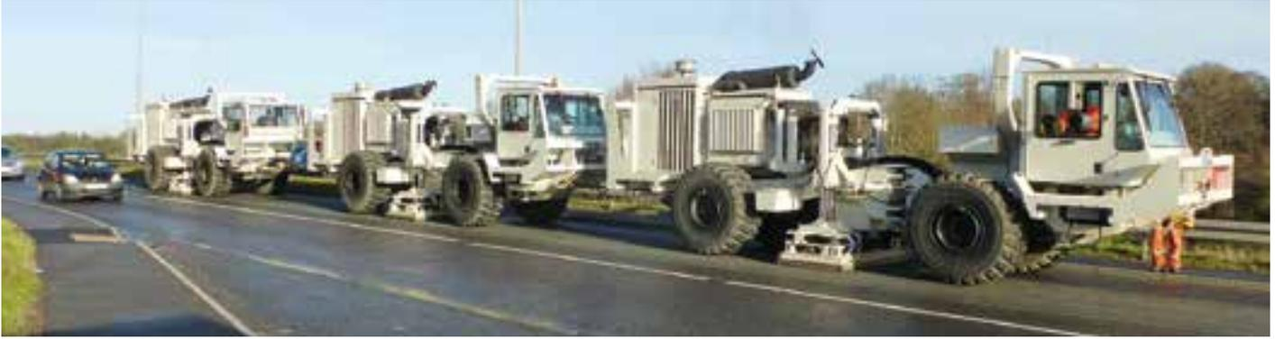
**Figure 2.** Vibroseis units working on a road in the Navan area.
