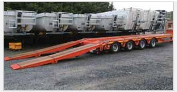
New Faymonville 4 axle 9ft wide, extendable, payload 60ton, double flip ramps, hydraulic legs under rear, out riggers, marker boards, ready to go.
