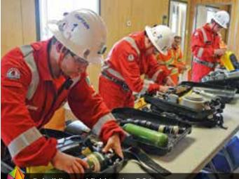
Rebuilding and field testing BG4s
