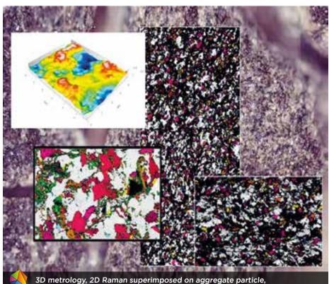
3D metrology, 2D Raman superimposed on aggregate particle,
