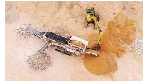
of soil and rocks. The soil has a high plasticity clay content which is stuck to the rocks. This type of clay clumps together instead of breaking up and is very problematic for regular vibratory screeners. The vibrating action liquifies the clay and makes it stick to the openings and blocks up the screens. Also, the rocks found in this mixture are as large as 800mm and are too big for regular vibratory screeners or recycling trommels.
