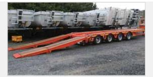
New Faymonville 4 axle 9ft wide, extendable, payload 60ton, double flip ramps, hydraulic legs under rear, out riggers, marker boards, ready to go.
