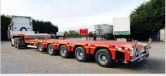
New Faymonville 5 axle step frame extendable low loader, 3 steer axles, front lift axle, auto greaser, option for hook on aluminium ramps or hydraulic ramps.
