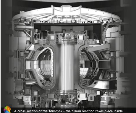
A cross section of the Tokamak – the fusion reaction takes place inside the 'D' shaped section, the machine weighs 23,000 tonnes of which 10,000 tonnes are magnets.
