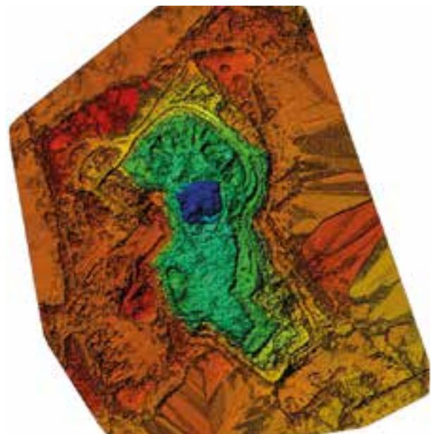
*Orthomosaic and the corresponding Digital Surface Model (DSM) of Kilmacow quarry.*
