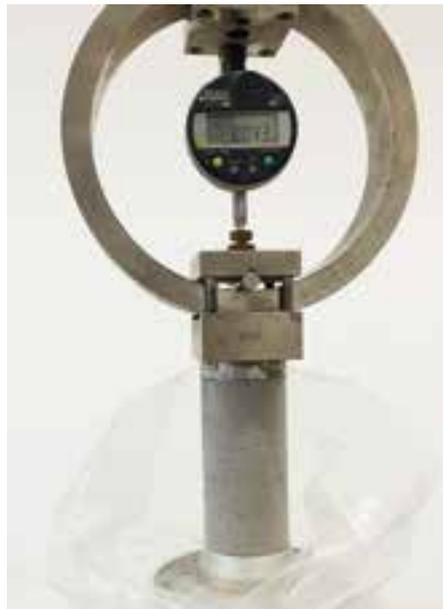
*Photograph of core of Pre-Treated APCr from the Duleek EFW plant undergoing unconfined compressive strength testing (UCS) at Queens University Belfast - August*
