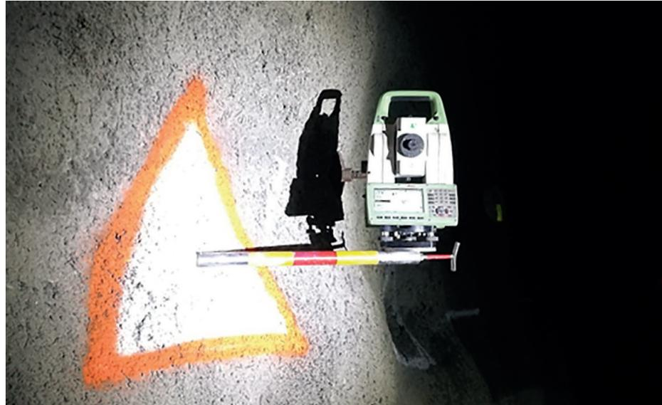
Figure 1: Leica TS16 Total Station mounted onto sidewall station.
