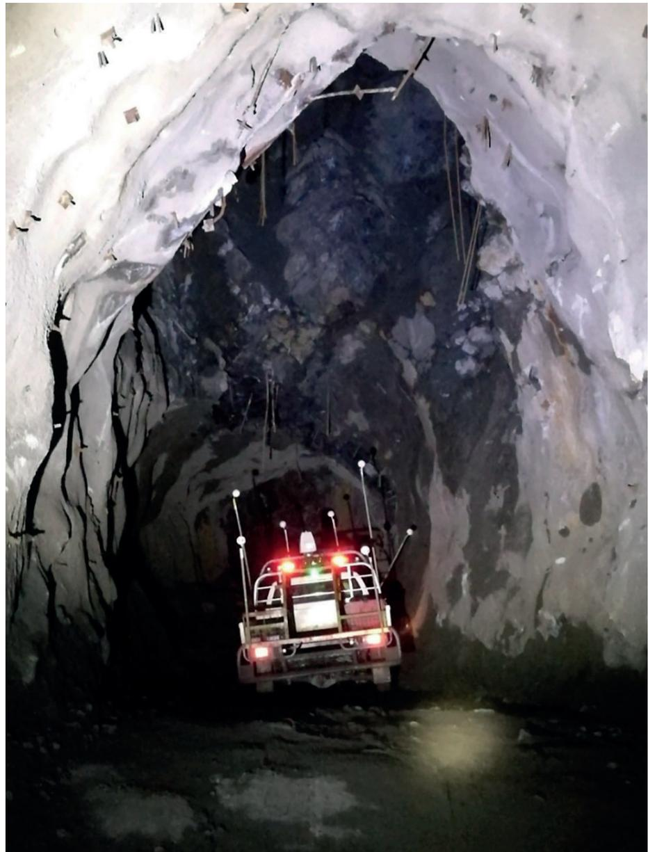
*Figure 3: Laser Scanning of stope using remotely operated vehicle with spherical targets visible.*
