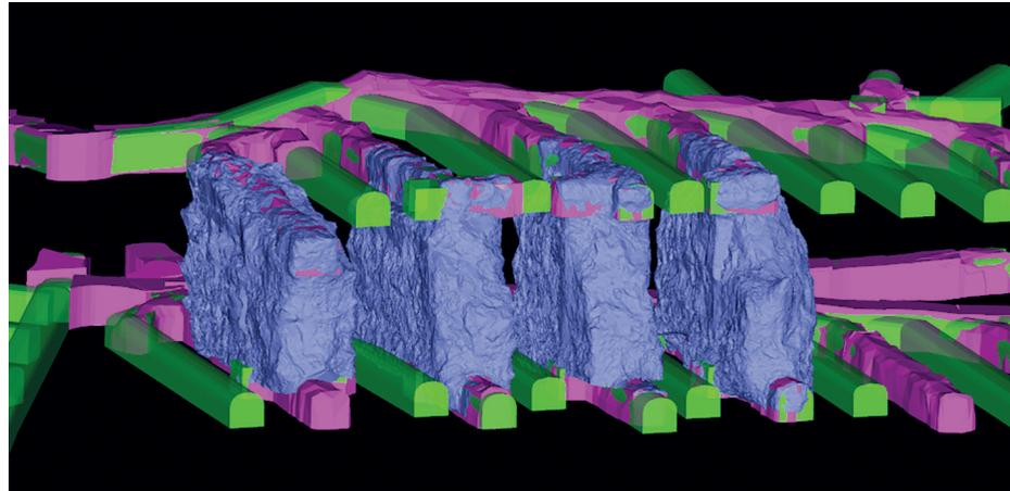
Figure 5: Deswik 3D view of slope scans (blue), survey development pickups (purple) and design solids (green) for hanging and footwall levels.
