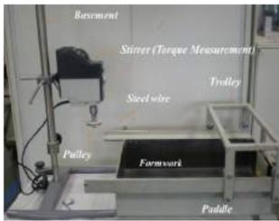
Figure n°2 – Placing Simulation Tool
