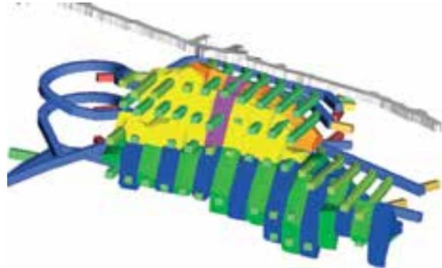
**Figure 3: Long Term designs for stopes and development. One of the current active blocks.**
