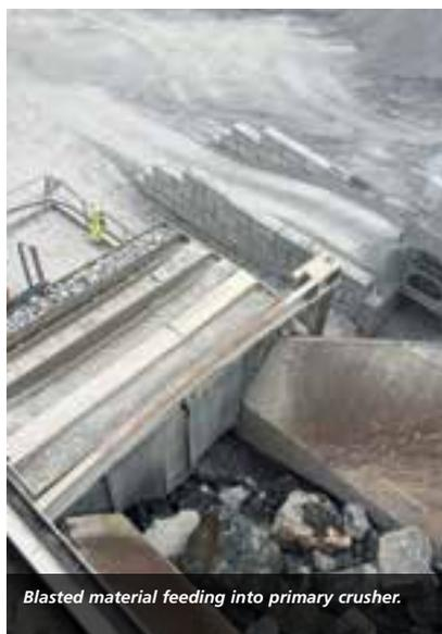
Blasted material feeding into primary crusher.
