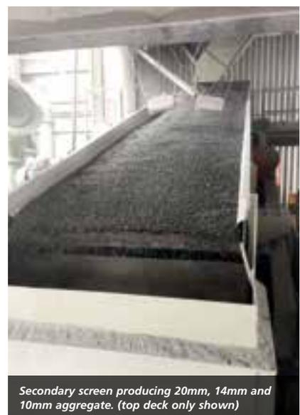
Secondary screen producing 20mm, 14mm and 10mm aggregate. (top deck only shown)
